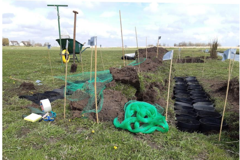
Image 1.1: Experimental setup and equipment. The right slot contains the pots with soil and the left slot contains the pots with dredge.
