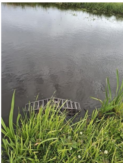
Figure 2: Funnel trap placement (also called “Finnish model” (610 x 315 x 250 mm)).
