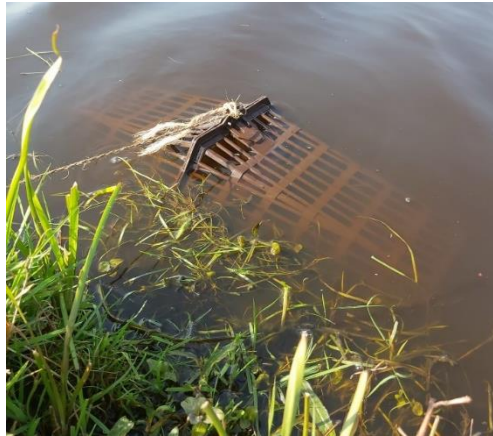
Figure 3: Positioning of the used crayfish traps to measure invasive crayfish abundance
